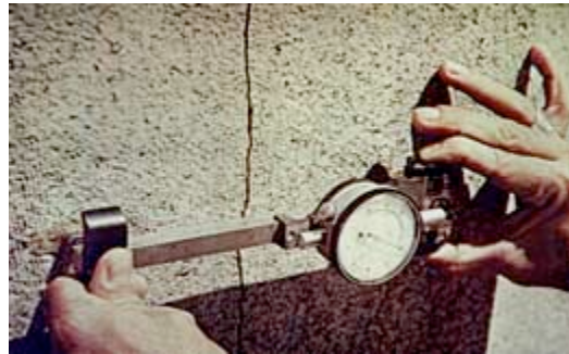
This crack is being measured. Structural cracking, whether static (nonmoving) or dynamic (moving) should be caulked to prevent water entry into the glazed architectural terra-cotta system. Photo: NPS files.
