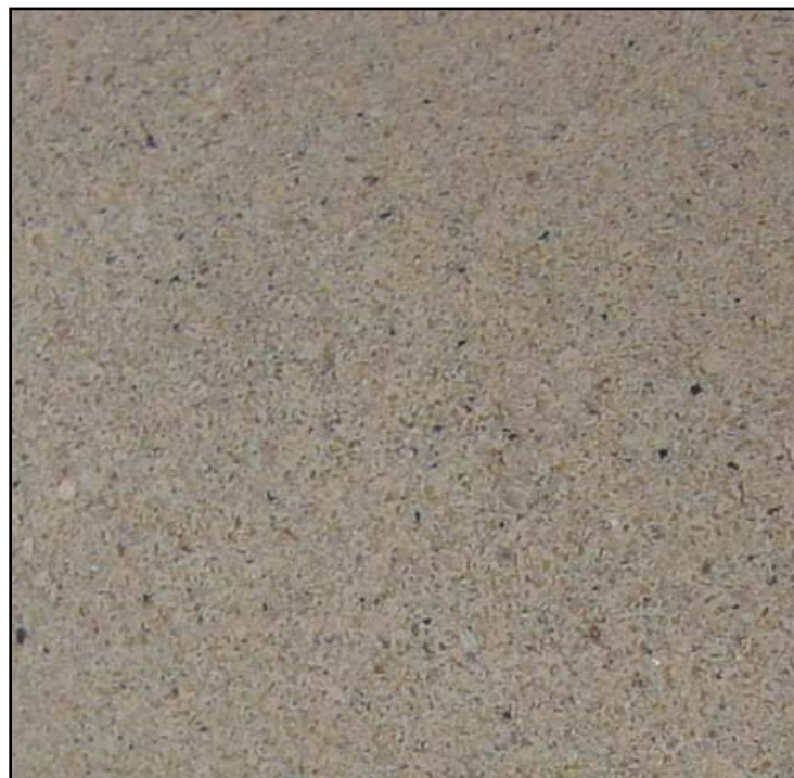
Close up of acid etched GFRC showing the grains of fine aggregate in the cement matrix.
