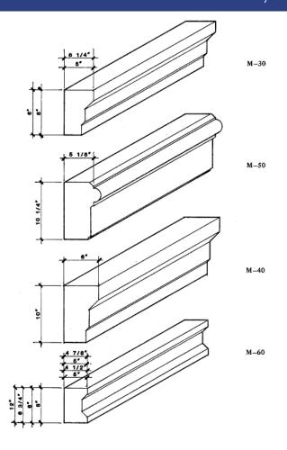
Some of the standard belt courses and band moldings. Custom shapes and sizes are available in both GFRC and Architectural Fiberglass.
