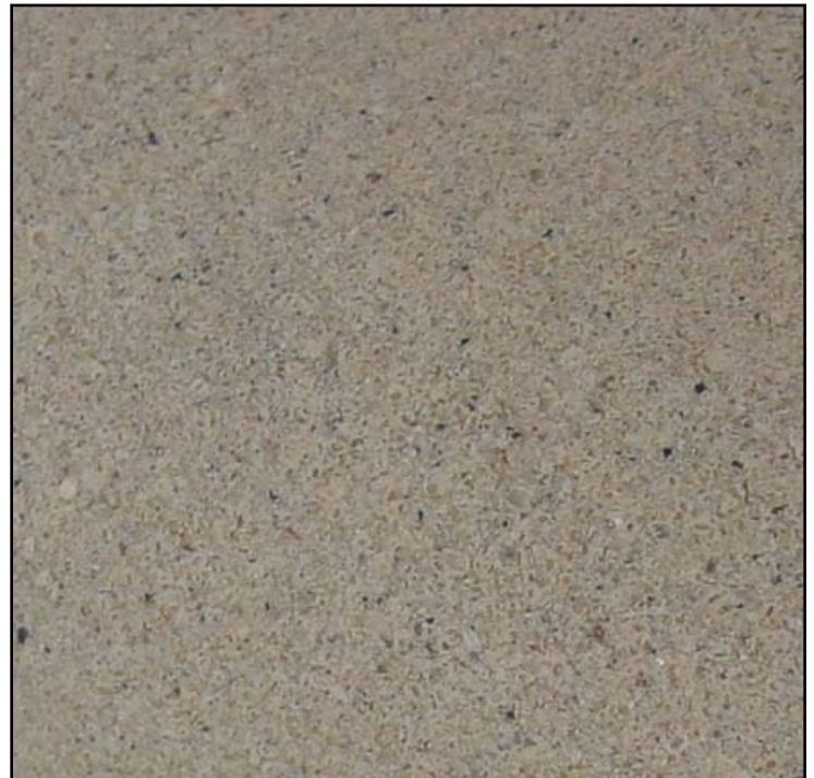
Close up of acid etched GFRC showing the grains of fine aggregate in the cement matrix.
