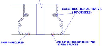
CONSTRUCTION ADHESVIE CAN BE USED WITH OR IN PLACE OF CAULK ALL JOINTS 3/8"+/-
