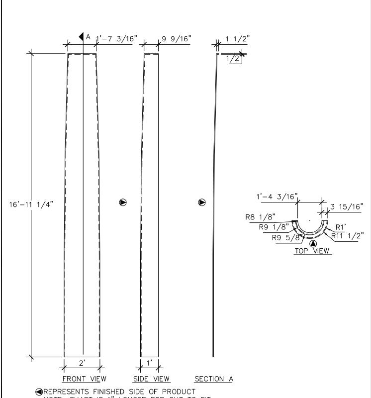
REPRESENTS FINISHED SIDE OF PRODUCT NOTE: SHAFT IS 1" LONGER FOR CUT TO FIT.
