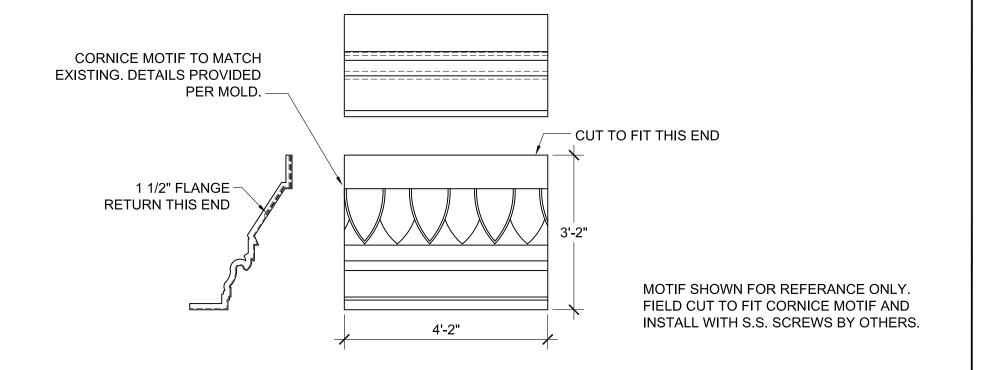
ALL RIGHTS RESERVED. THIS DRAWING IS PROPERTY OF STROMBERG ARCHITECTURAL PRODUCTS INC. AND MAY BE USED ONLY WHEN UTILIZING STROMBERG ARCHITECTURAL PRODUCTS. STROMBERG ARCHITECTURAL PRODUCTS INC. GENERAL TERMS AND CONDITIONS APPLY AND ARE INCORPORATE HERE IN BY REFERENCE. THIS DETAIL MAY NOT APPLY TO ALL CONDITIONS AND CONSTRUCTION SITUATIONS.
