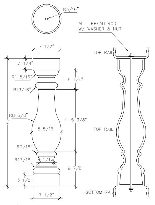
ASSEMBLE EIGHT (8) BALUSTERS IN SHOP. EACH TO HAVE FULL TOP AND BOTTOM WITH 9/16" DIA. HOLE IN CENTER.
